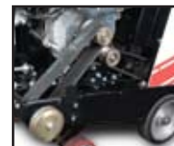
7 3VX V-belt drive from engine to blade shaft
